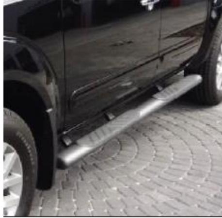
**Step 4.** Carefully place step into position on OE mounting studs.
