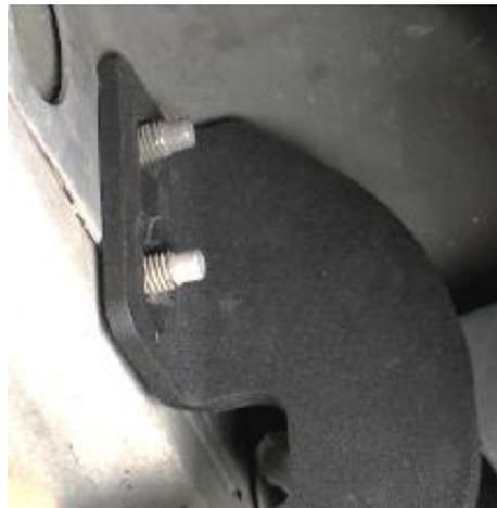
**Step 6.** Begin tightening nuts in an alternating pattern. ***NOTE: Over tightening could strip or break studs.*** Tighten to 20 (ft/lbs) torque to secure to vehicle.
