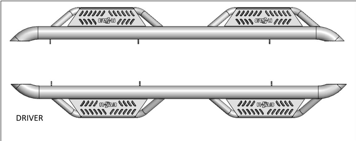
**Step 2:** Install the (x6) mounting brackets to each attachment point on the main tube using the supplied M10x25 carriage bolts, M10 hex nuts and leave loose for now.
