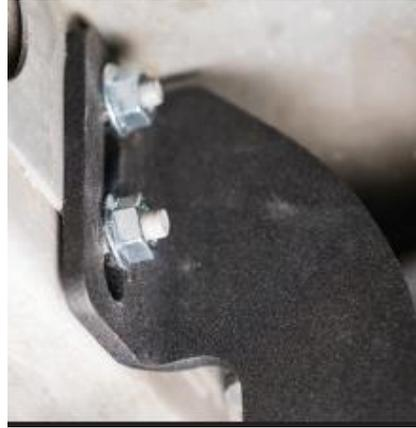
**Step 7.** After final adjustment, tighten all three brackets at the main tube.
